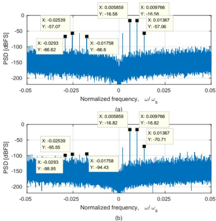
HD<sub>3</sub> and IM<sub>3</sub> correction blocks operated successfully.
