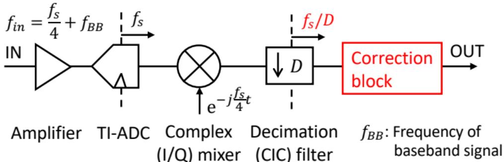
Digital correction method for third-order nonlinearity of TI-ADCs in direct-RF sampling receivers:
