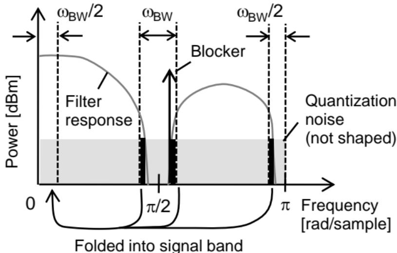
The CIC filter needs to reduce the folded noise and blockers to obtain the required output SNR ( $SNR_{out}$ ).
