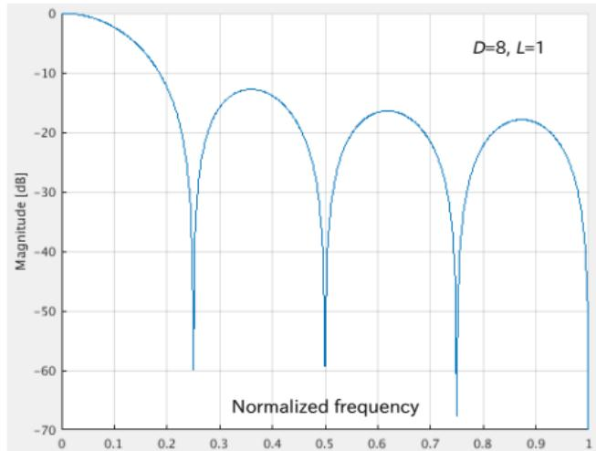
$$|H_{CIC}(\omega_1 \pm \omega_{BW}/2)| \approx |H_{N,CIC}(2\pi/D_N \pm D_1 \cdots D_{N-1}\omega_{BW}/2)|$$
