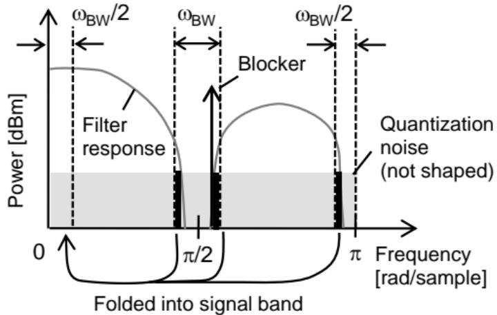
Noise power around  $\omega_k$  ( $P_{n,k}$ ) and total noise power folded into  $\omega_{BW}$  ( $P_n$ ):
