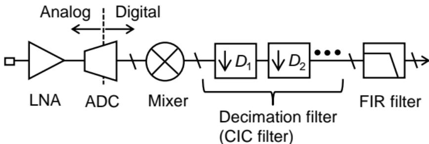
LNA: Low-noise amplifier, ADC: Analog-to-digital converter,
